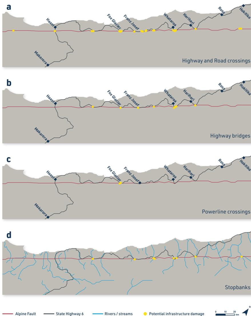
**Figure 4:** Sites of potential infrastructure damage caused by ground surface rupture of the Alpine Fault, between the Cascade and Kokatahi rivers.
